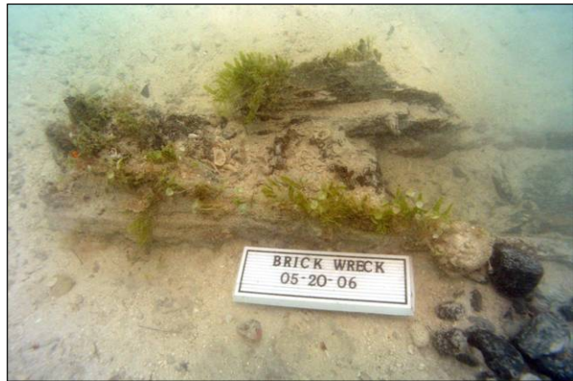
Figure 17. Stern assembly (from right to left): inner sternpost, sternpost, and iron strapping or lower gudgeon
